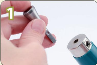
**1** Insert the inverted mandrel into the base of the Conetastic Tool (sold separately) with flat side of the mandrel shank aligned with the set screw.
