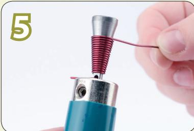
**5** Continue turning the tool to wrap the wire around the mandrel.
