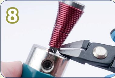
Use the flush side of a cutter to snip the wire at the bottom to release it from the hole.
