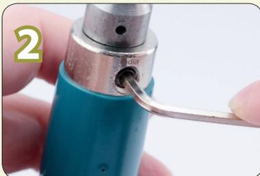
**2** Use an Allen Wrench to tighten the Inverted Mandrel into place.
