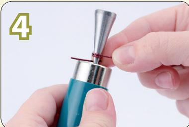
**4** Holding and guiding the wire with your fingers, turn the Conetastic Tool to wrap the wire around the mandrel.
