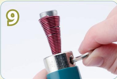
Use the Allen Wrench to loosen the mandrel and remove it from the Conetastic Tool.
