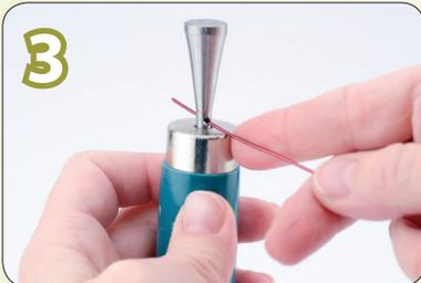
**3** Insert wire into the hole at the base of the mandrel to secure the wire for wrapping.
