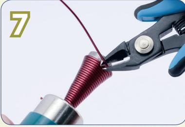
Use the flush side of a cutter to snip the end of the wire.
