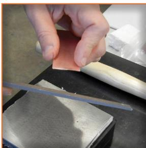
4. Clean metal with Penny Brite® (our favorite) or an abrasive cleaner and scrubbie. The metal must be very clean. Water will sheet off (not bead up) on the surface when it is truly clean.
