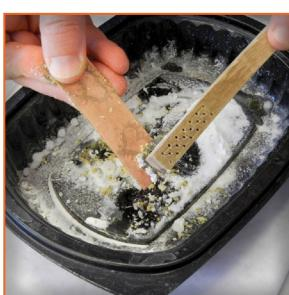
15. Patina the metal with an oxidizing agent to really bring out the definition in your design. Polish with steel wool or a wire brush. If you're doing a large batch of items, or you hate the task of polishing, use a tumbler.
