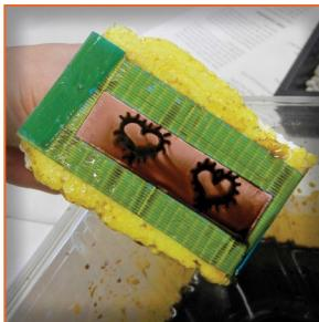
14. Scrub metal clean in a sink or tub of water. Use baking soda to neutralize the acid if desired. Some people use a weak ammonia bath to really make sure the acid is removed.
