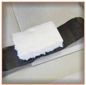
8. Wrap the duct tape around the styrofoam block with the sticky side out.
