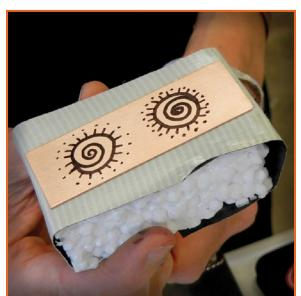
12. Allow to float for 30-90 minutes, depending on depth of etch desired. Nickel silver tends to take longer than copper or brass because it contains just 65% copper (the rest is nickel and zinc).
