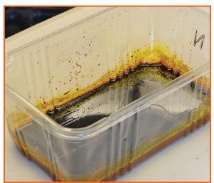
11. Attach metal to the float boat. Suspending the metal into the bath with tape is another option. Just make sure the metal is submerged yet not touching the bottom of the container.
