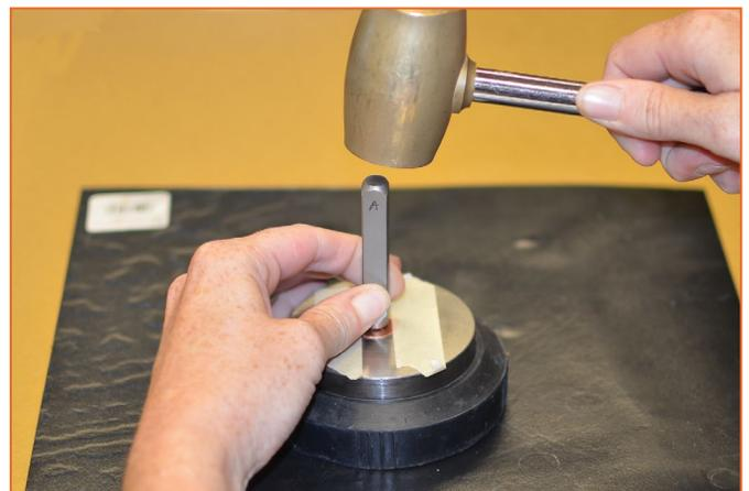
2. Place the letter stamp in the center, straight up and down perpendicular to the metal. Hit the stamp directly with one firm blow.
