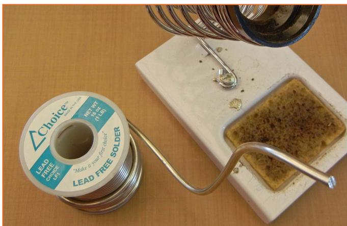
*Shaping the solder coil into a snake makes it easier to feed onto your soldering iron*
