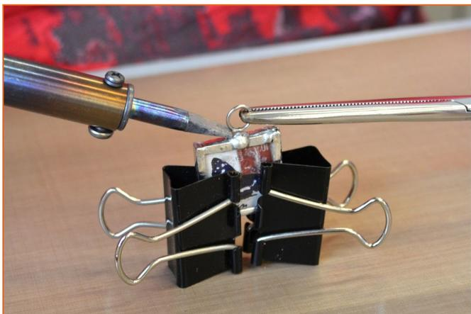
*Using hemostat to hold the jump ring in place while melting the solder blob with the iron.*
