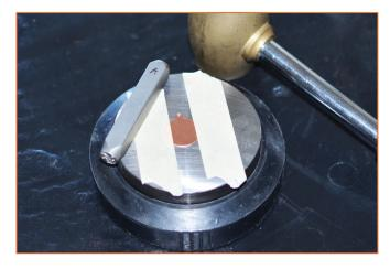
1. Tape your metal blank to your steel block or anvil to keep it from sliding or moving.
