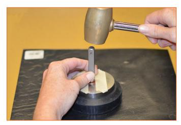
2. Place the letter stamp in the center, straight up and down perpendicular to the metal. Hit the stamp directly with one firm blow.
